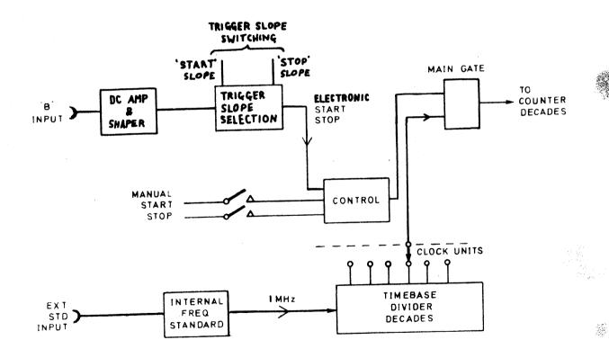
Fig. 2.3 Time Interval - Single Line
