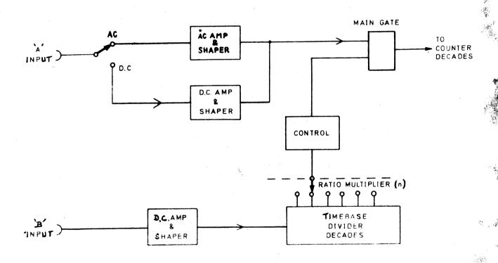
Fig. 2.5 Ratio Measurement
