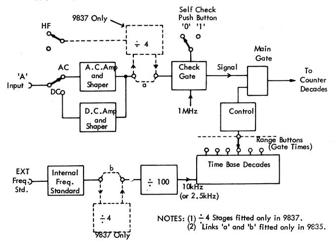
Fig. 2.1 Frequency Measurement
