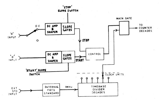
Fig. 2.4 Time Interval - Double Line
